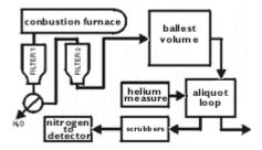
To use LECO's combustion analyzer, 1-4 g of sample is placed in a reusable ceramic boat on a 49-position autoloader. The boat automatically moves into a furnace where it combusts in a pure oxygen atmosphere. moisture is removed from the combustion gases via a thermo-electric cooler before being routed into a ballast. The gases are given time to equilibrate before an aliquot is taken. Interfering gases are removed and nitrogen is detected by thermal conductivity. The analysis takes five minutes.
