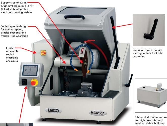
Automatic pulse feed rate with load control maximizes sectioning efficiency without burning samples
